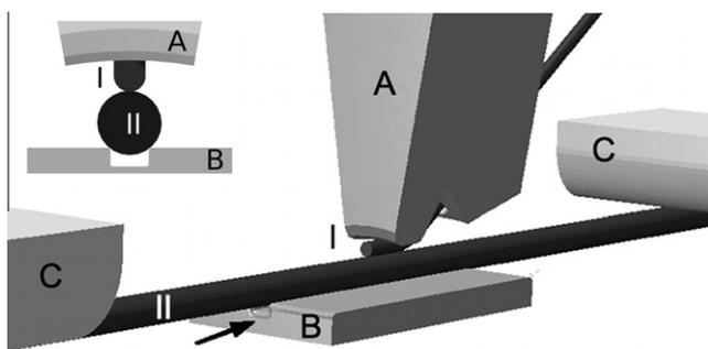
**Fig. 1.** The wire-to-wire bonding process. The base wire (II) is attached to the grooved substrate (B) with clamps (C). The tension created by the clamps together with the support from the groove (arrow) in the substrate keeps the base wire firmly in its position during the bonding process. The standard bonding wedge (A) bonds the upper wire (I) to the base wire. The insert (top left) shows the front view of the bond location.
