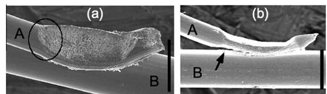
**Fig. 3.** SEM images of two wire-to-wire bonds. A 25  $\mu\text{m}$  wire (A) is bonded to the 50  $\mu\text{m}$  base wire (B). (a) The bond shape is visible. No cracks in the encircled neck area. (b) The unbonded area under the neck is shown with an arrow. The black size bar is 50  $\mu\text{m}$ .
