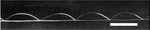
**Fig. 4.** Multiline 2-wire tether produced using wire-to-wire bonds. The loop height is 2.5 mm and the loop length is 12 mm. White scale bar is 10 mm long.
