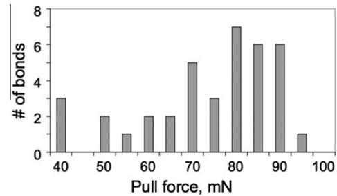
**Fig. 2.** Measured pull forces for 38 wire-to-wire bonds.
