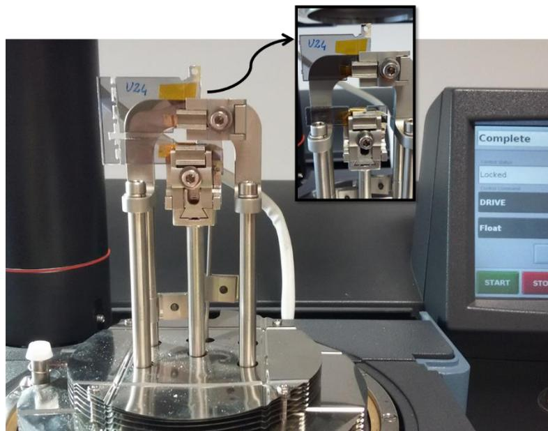
Figure 71: Sample installed in the DMA before and after the tensile test.
