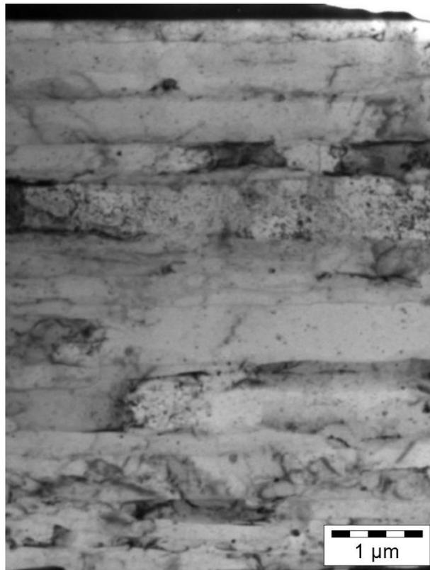
Figure 101: Grains oriented in the drawing direction in sample tested at 100 °C (test 138).
