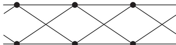
**Fig. 2.** Model of four-line micrometeoroid-resistant “Hoytether” [6]. The structure as a whole does not break if and when micrometeoroids cut some wires. The structure width is  $\sim 3$  cm and the wire thickness  $\sim 25 \mu\text{m}$ . Sites where wire-to-wire bonding is needed are marked with dots.
