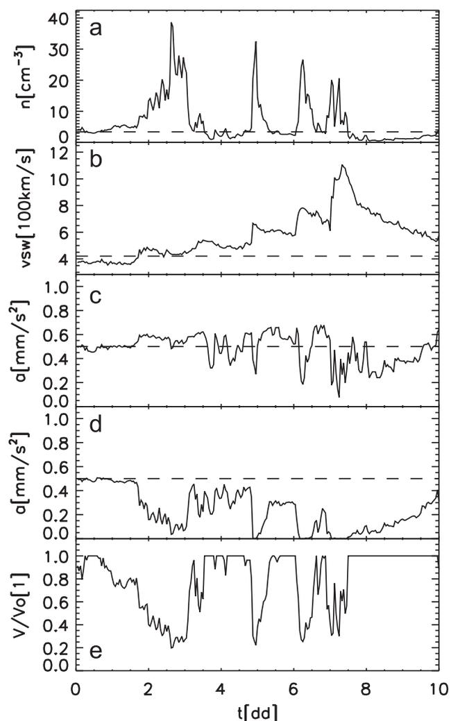
Fig. 3. Solar wind density (a) and speed (b), resulting electric sail acceleration with 40 kV (c) and 10 kV (d) maximum voltage, as well as voltage variation compared to maximum (e), over a 10-day period when solar wind showed large variations [8].
