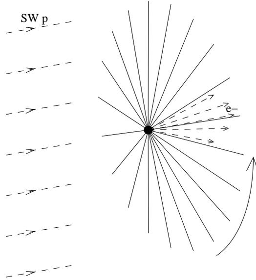
Figure 1. Schematic presentation of the electric solar wind sail deep-space propulsion method.
