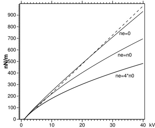
Figure 5. The approximate thrust per length, Eq. (4) (dashed) with more accurate results from Janhunen (2009b), with different values for average electron density inside the electrosphere.  $R = 100$  m was assumed.
