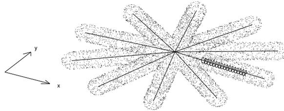
Figure 3. Starfish-shaped potential structure of multi-tether electric sail and typical electron orbit around a tether
