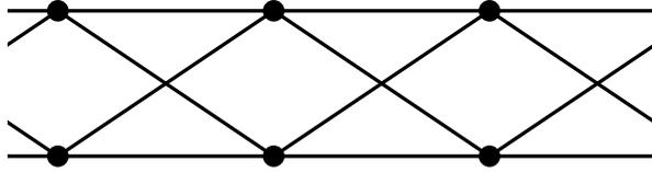
Figure 4. A four-wire Hoytether. Wire bonding sites are shown by dots.
