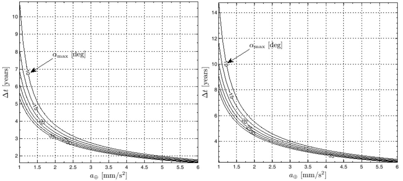
**Fig. 5.** Optimal time to reach Uranus (left) and Neptune (right) flyby, as a function of electric sail acceleration at 1 AU and for a few values of the maximum cone angle  $\alpha_{\max}$ .
