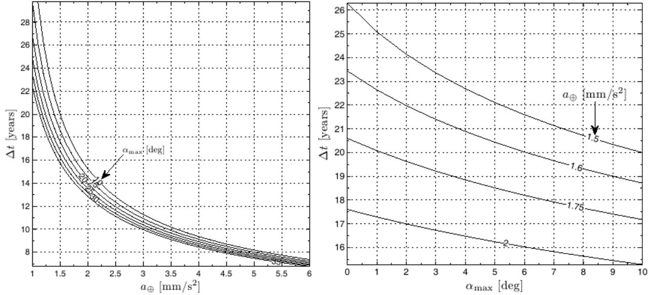
**Fig. 1. Left: Optimal flight time to 100 AU as a function of the electric sail acceleration at 1 AU for different values of maximum cone angle  $\alpha_{\max}$ . Right: Case of small  $\alpha_{\max}$ , with roles of  $\alpha_{\max}$  and acceleration interchanged in the plot.**
