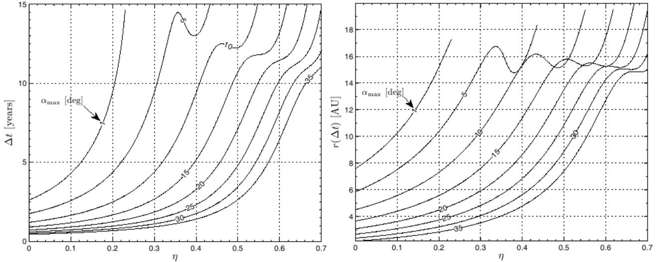
**Fig. 4. Left: Time to reach the escape trajectory from the Solar System using a complete thrust model as a function of the payload fraction  $h$  for 20 mm wire diameter and for discrete values of the maximum cone angle  $\alpha_{\max}$ . Right: Sun-spacecraft distance (in Astronomical Unit) where escape condition is reached.**
