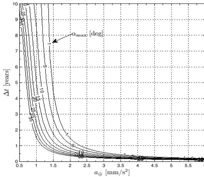
**Fig. 3. Time to reach an escape trajectory from the Solar System as a function of electric sail basis acceleration  $a_A$  and for discrete values of the maximum cone angle  $\alpha_{max}$ .**
